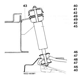
2 Release left-hand engine shock absorber (straightahead) at top and unscrew bolt which holds engine bearer.
